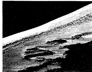
Fig. 10 Thermal erosion downstream from isolated pieces of hard coat (magnification = 12x).
